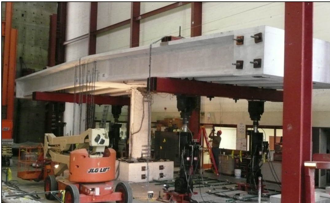
Figure 6.34: Displaced Test Unit at -6 in. of Displacement
