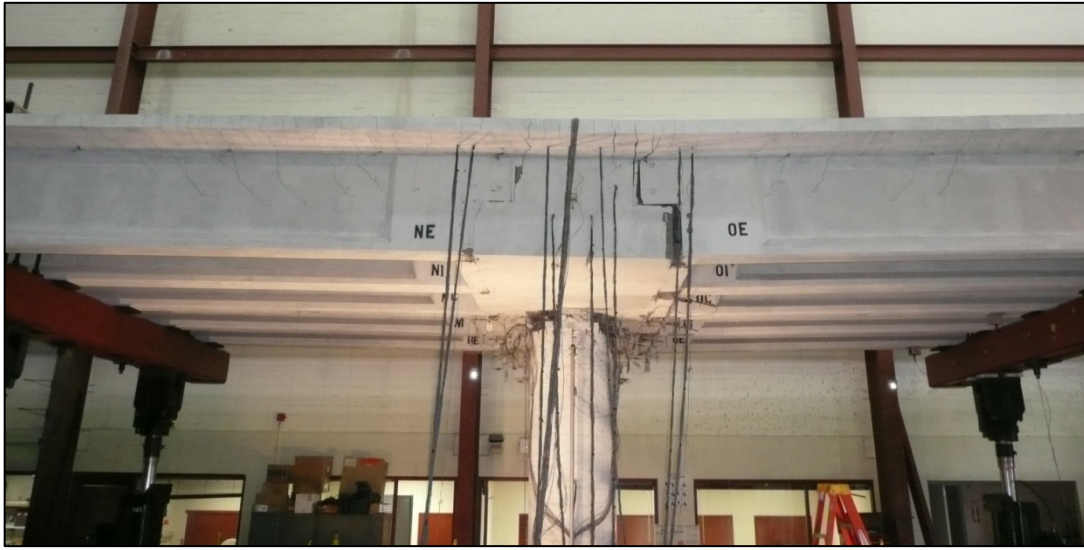
Figure 6.35: Overall Response of Test Unit at +3 in. of Vertical Displacement
