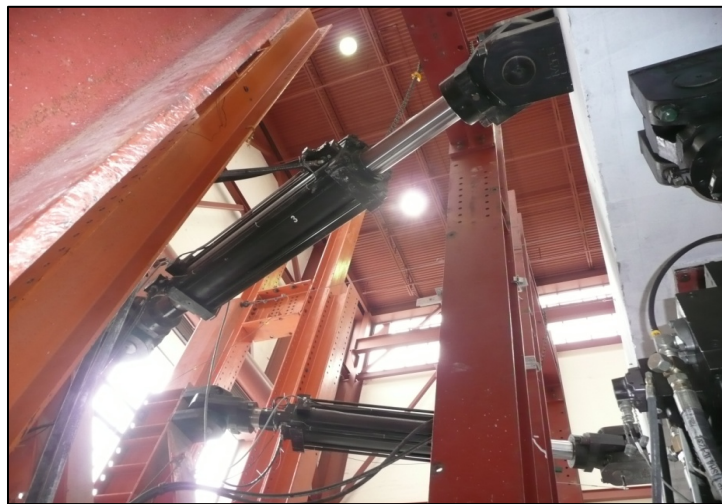
Figure 6.1: Horizontal Actuator Configuration Used During Phase 1 Testing at Each Abutment
